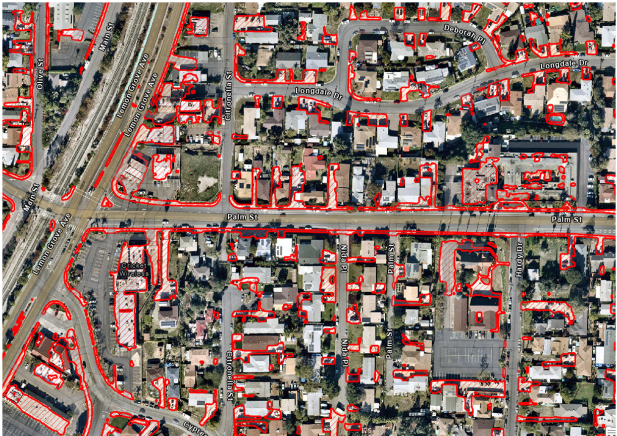
Example of third-party vendor machine learning concrete asset extraction displaying concrete ground covering.
