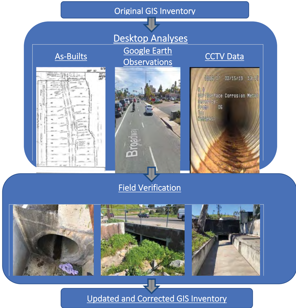
Figure 2-2: Corrections to GIS Inventory Flowchart
